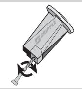
Unscrew pin and remove to complete the installation.
