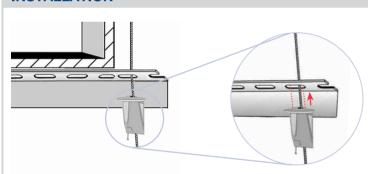
Gripple Trapeze slots into the configuration of the channel.
